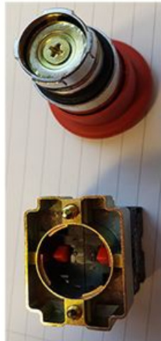
E-Stop actuator and dual block housing
