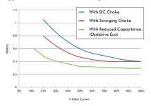
It can be clearly seen that the reduced DC link capacitance significantly reduces the total harmonic distortion at full load, and has a much greater benefit at part load compared to a conventional DC choke or swinging choke. This results in reduced overall input current and reduced transformer heating effect.
