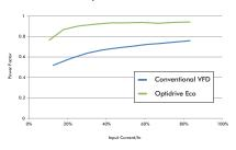
Optidrive Eco offers improved power factor over conventional VFDs under all loads.
