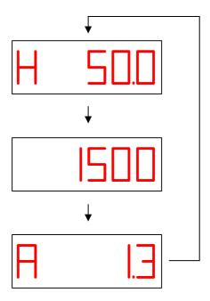
**Note:** When parameter P-10 is set, the following speed parameters will be displayed in RPM rather than Hz:
