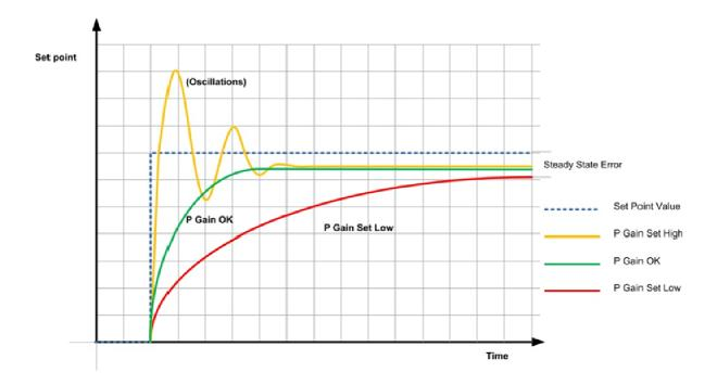
The Integral (I) term in a PI function samples the error present over a given time and takes an average of those values, hence the affect on the system is based on the accumulation of recent errors rather than the current or existing error. The I term is used to eliminate the steady state error (caused by only applying P term) and it adds
