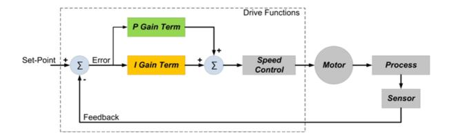
The proportional (P) term in a PI function is simply a multiplier for the error signal and is the easiest to understand and adjust. Hence the P term directly affects the size of the error value seen by the PI controller and how quickly the drive output responds. If the P gain value is set too low then the drive will take more time to modify its output and
